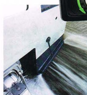
Zipwake's through-hull wires are sensibly sited above the waterline
