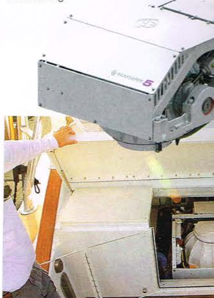
The new Seakeeper 5 is so small and light that boats benefit from gyro stabilisation
